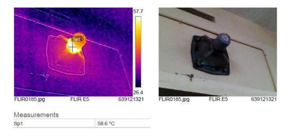
3. Thermal image of ceiling fan – The temperature of the ceiling fan is found to be 70.1 <sup>0</sup>C. The high temperature might be because of its life period. It is recommended to replace such oldest fan to save considerable amount of energy.
